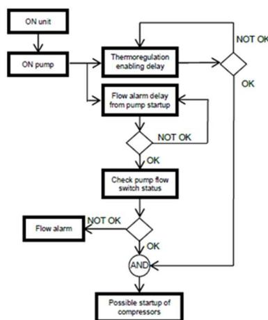
Note: that the thermoregulation is not enabled until stable flow conditions are detected after the flow alarm delay from pump startup. This is to prevent the starting up of compressors when there is not yet certainty of the water flow presence.
